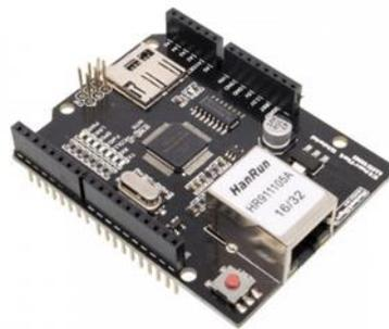
**Figura 3-18: Shield Ethernet**
